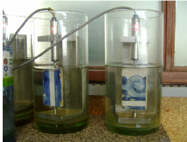
Figure 2 - Moisture expansibility measurement set-up.
